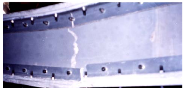
Fig. 9. Tension failure for GFRP I-beams
